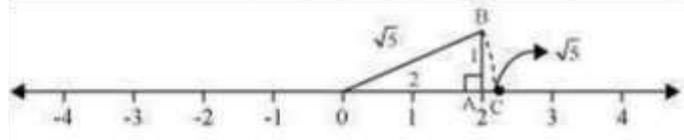
Mark a point 'A' representing 2 on number line. Now, construct AB of unit length perpendicular to OA. Then, taking O as centre and OB as radius, draw an arc intersecting number line at C.
